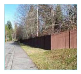
Regular sealer applications (stain/paint, etc.) on the timeline indicated are strongly recommended for appearance and protection of wood fencing. Remove any contact with ground and surrounding landscape and sprinkler patterns, repair as needed and clean prior to sealer application. Life of finish will vary depending upon surface preparation, material quality, application method and weather conditions.
